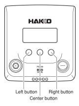
HAKKO FX-100 has 3 operation buttons. The operation executed by each button varies depending on what is on the display screen. The operation for each button is indicated at the bottom of the screen. Select the button according to the indication.
