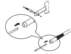
2. Hold the head part of the T31 series tip (not included) with the heat resistant pad and insert the tip into the handpiece. Push until the tip stops
