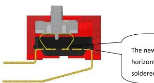
The new contact structure of moving horizontally makes NDA available to be soldered both ON/OFF positions.
