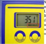
When the MAX HOLD function is on, the maximum temperature is constantly displayed on the LCD.
