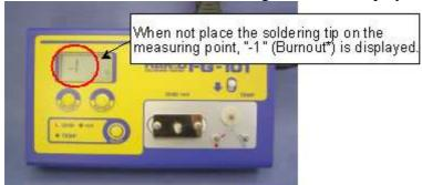
4. Press the AUTO ZERO button and wait until the display returns to normal status. The correction value generated by the AUTO ZERO function is recoreded in the main unit. It remains in the memory even when the power is turned OFF, and is valid also in the next measurement.
