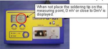
4. Press the AUTO ZERO button and wait until the display returns to normal status. The correction value generated by the AUTO ZERO function is recorded in the main unit. It remains in the memory even when the power is turned OFF, and is valid also in the next
