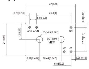
Case No.IRM03 Unit:mm[inch] Tolerance:±0.5[±0.02] unless otherwise specified
