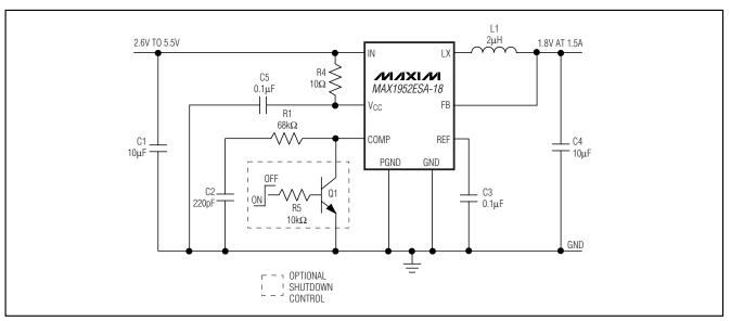
Figure 2b. MAX1952 Fixed-Output Typical Application Circuit
