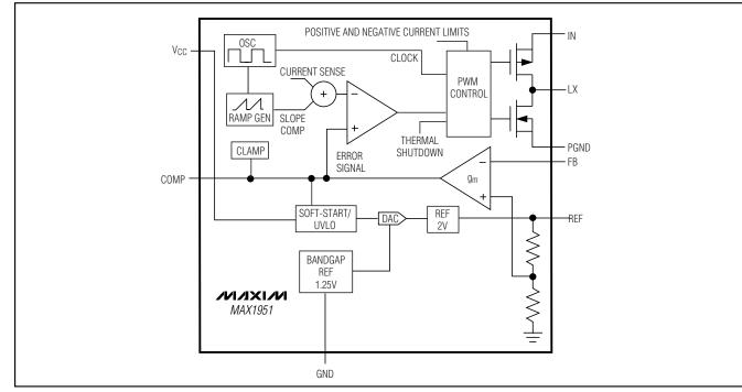
Figure 1. Functional Diagram
