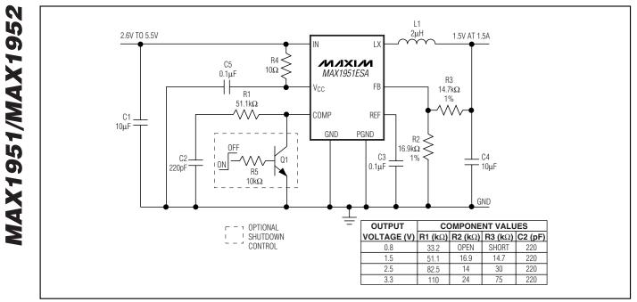
Figure 2a. MAX1951 Adjustable Output Typical Application Circuit
