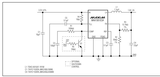
Figure 2c. MAX1951 Typical Application Circuit with 2A Output
