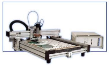
The Bungard CCD/MTC is a high quality Computer Controlled Drilling machine with Automatic Tool Change. It allows direct processing of Excellon/Sieb&Meyer drill data or HP/GL plot data for PCB production (drilling, milling, isolation routing, dispensing) and milling/routing of plastics, aluminium or other metal panels.
