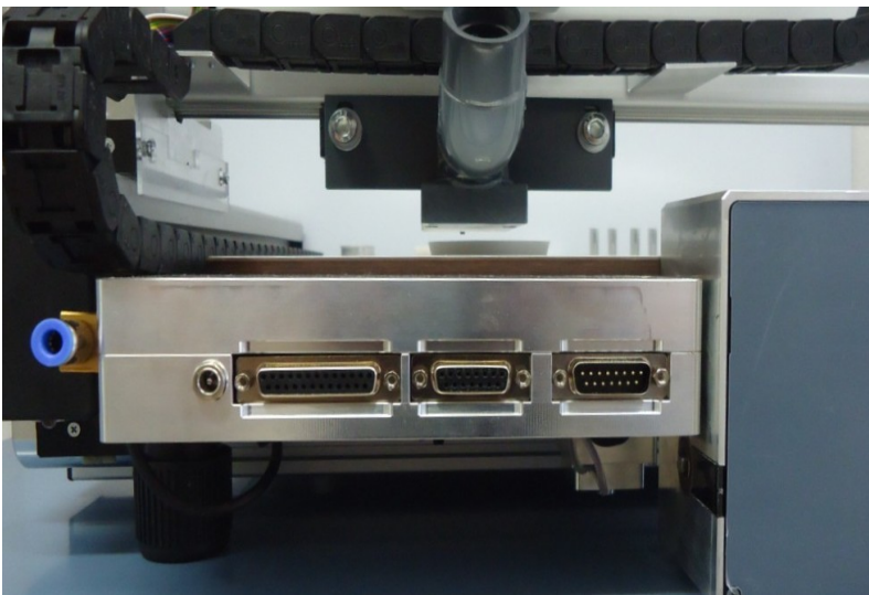
5: ATC motor connection box
