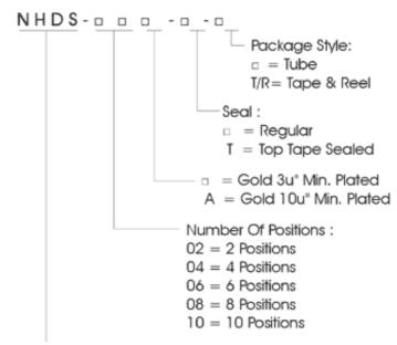
New Half Pitch Type Dip Switch (H = 1.6 mm)
